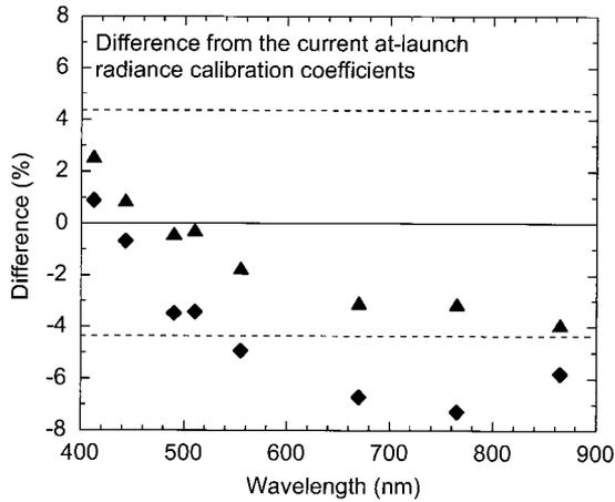
Fig. 4. Percent differences from the 1997 prelaunch calibration coefficients for SeaWiFS. The 1997 prelaunch coefficients are the current at-launch calibration coefficients for the instrument. The dashed lines give the estimated uncertainty ( $k = 1$ ) for the on-orbit calibration of SeaWiFS. The differences of the on-orbit radiance calibration coefficients are shown as diamonds. The differences of the 1993 laboratory calibration coefficients are shown as triangles.
