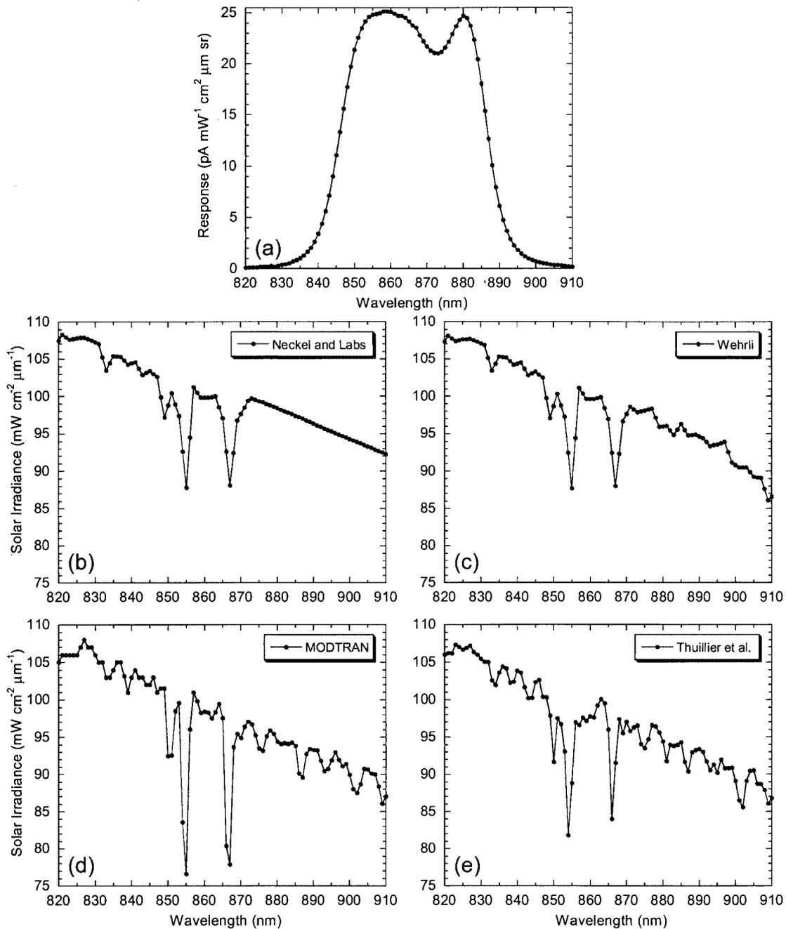
Fig. 2. SeaWiFS band 8 spectral response and irradiances from four solar models. The values in each panel are given at 1-nm intervals from 820 to 910 nm. (a) The band 8 spectral response is in units of picoamperes from the photodiode detector per unit spectral radiance.<sup>15</sup> The solar irradiances come from the models of (b) Neckel and Labs,<sup>14</sup> (c) Wehrli,<sup>16,17</sup> (d) MODTRAN,<sup>18,19</sup> and (e) Thuillier *et al.*<sup>20</sup>
