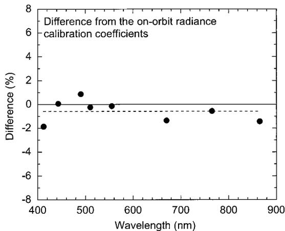
Fig. 3. Percent differences from the on-orbit radiance calibration coefficients for SeaWiFS. The differences of the prelaunch SRBC coefficients are shown as circles. The dashed line gives the average value for the eight differences. Both sets of coefficients use the solar irradiance model of Thuillier *et al.*<sup>20</sup> in their calculation.
