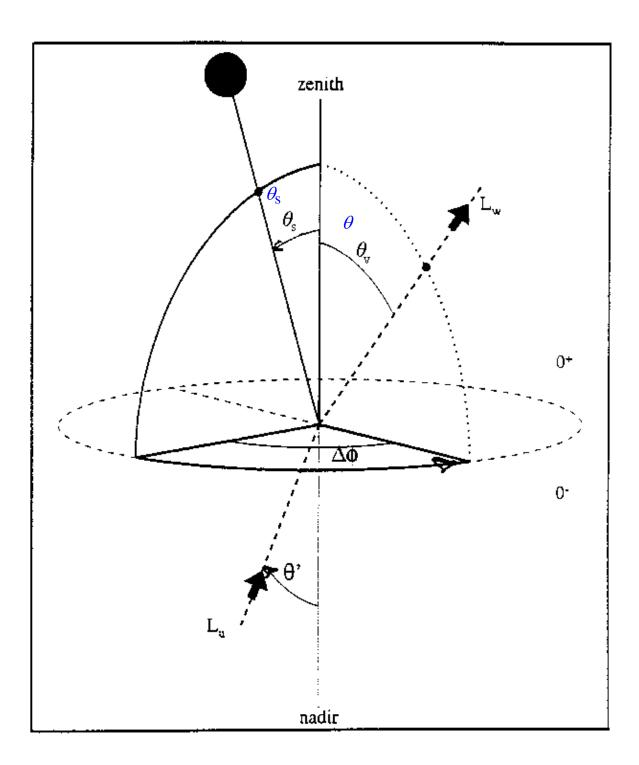
$L_{u} = \text{in-water upwelling radiance}$  $L_{w} = \ll \text{water-leaving} \gg \text{radiance}$  $L_{w} = L_{u} \frac{1 - \rho_{F}(\theta')}{n^{2}}$
