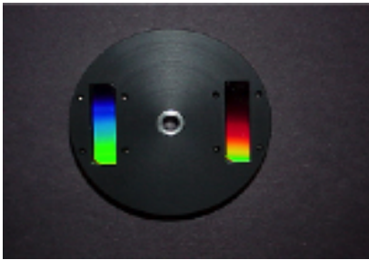
Figure 3. Filter wheel of ac-s.
